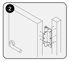
Easy 2 step installation process. Step 1, insert allen key into head and turn to set tension reinsert pin. Step 2, screw or rivet hinge to door and door jamb. Easy. You're done.
