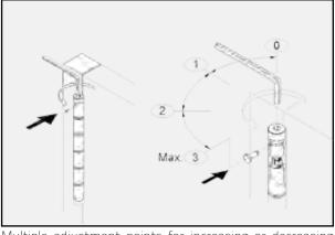
Multiple adjustment points for increasing or decreasing the spring's tension. Simple function, pull pin, turn head with allen key and replace pin. No need to remove door
